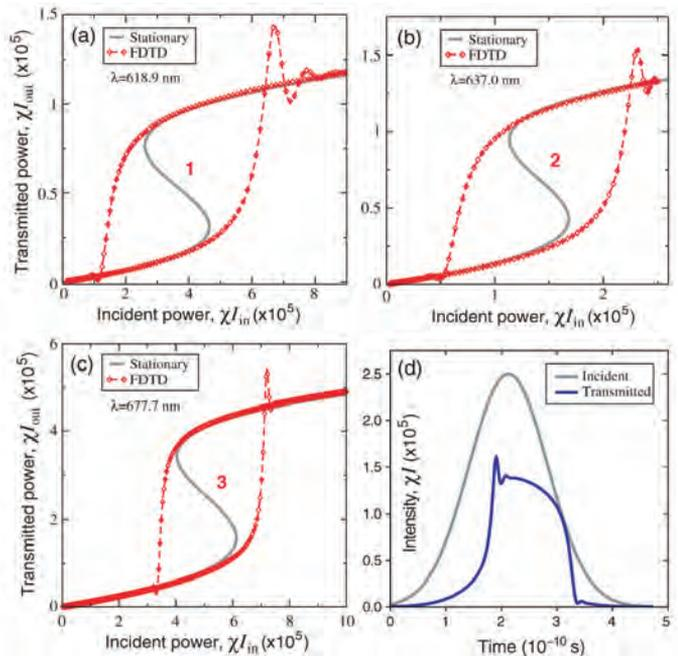
**Fig 3:** Stationary and FDTD simulations showing hysteresis loops in the output versus input power dependence for three selected resonances. Panel (d) shows deformation of the transmitted Gaussian pulse corresponding to the hysteresis switching.
