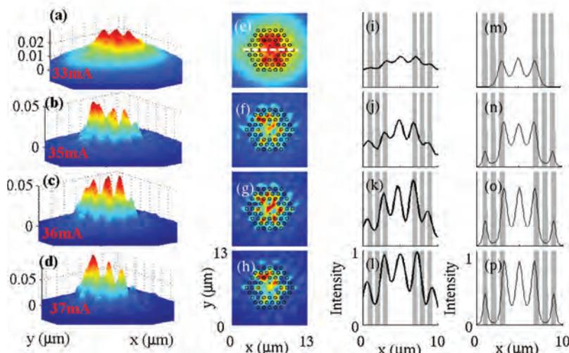
**Fig 2:** Experimental demonstration of soliton lattices with three-dimensional and two-dimensional NSOM images (first and second rows). The injection currents are (from top to bottom): 33, 35, 36, and 37 mA, respectively. The third row shows the mode profiles along the horizontal direction, i.e., along the dashed line in (e). The shaded areas mark a periodic lattice.
