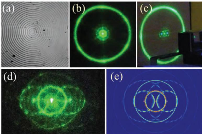
**Fig 4:** (a) Microphotograph of the Z surface of the annularly periodically poled structure. (b) Experimental image of nonlinear diffraction with a single fundamental beam and (c) with two beams crossing in the center of the structure. (d) Magnified central part of the pattern (c). (e) Numerically calculated second harmonics emission from the virtual-beam nonlinear diffraction process.
