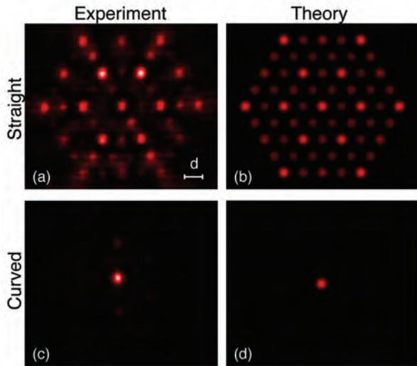
**Fig 1:** (a) Experimentally measured and (b) numerically calculated output beam profiles for the hexagonal lattice created by straight waveguides. (c) Experimentally measured and (d) numerically calculated output beam profiles for the hexagonal lattice created by periodically curved waveguides.
