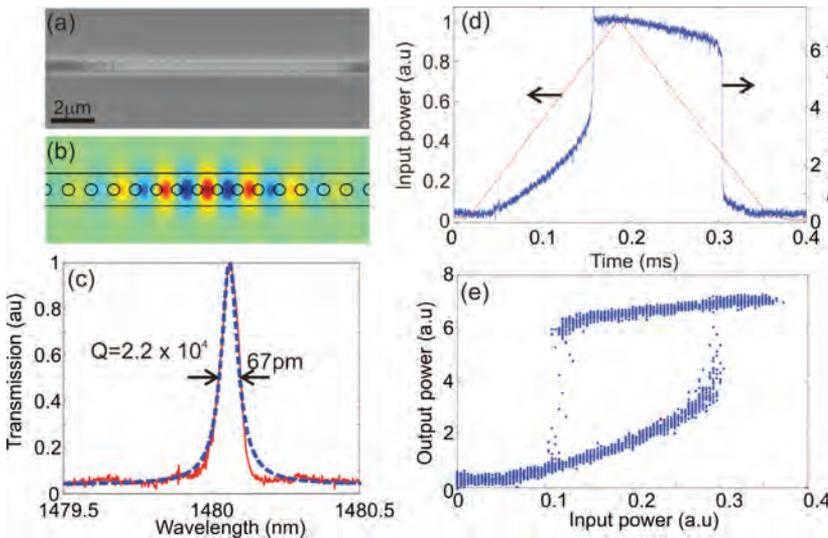
**Fig 3: (a) SEM image of a fabricated chalcogenide wire nanocavity. (b) Calculated  $E_y$  field profile of the cavity mode. (c) Measured resonance transmission spectrum (solid red curve), and fitted Lorentzian with  $Q = 2.2 \times 10^4$  (dashed blue curve). (d) Transmitted power (blue curve) while sweeping the input power up and down (red curve) with a CW laser detuned just above the resonance wavelength. (e) Bistability curves showing output power as a function of input power.**
