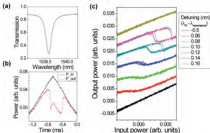
**Fig 1: (a). The resonance spectrum for the thermal bistable switching measurement. Resonance linewidth (FWHM) = 0.148nm,  $\lambda_0 = 1539.597\text{nm}$  (b): Input and output power plotted as a function of time for a detuning of 0.14nm. Switching times were:  $t_{\text{rise}} \sim 63\mu\text{s}$ ,  $t_{\text{fall}} \sim 93\mu\text{s}$  (c): Output power against input power for a range of detuning. Thermal hysteresis was observed for sufficiently large detuning.**
