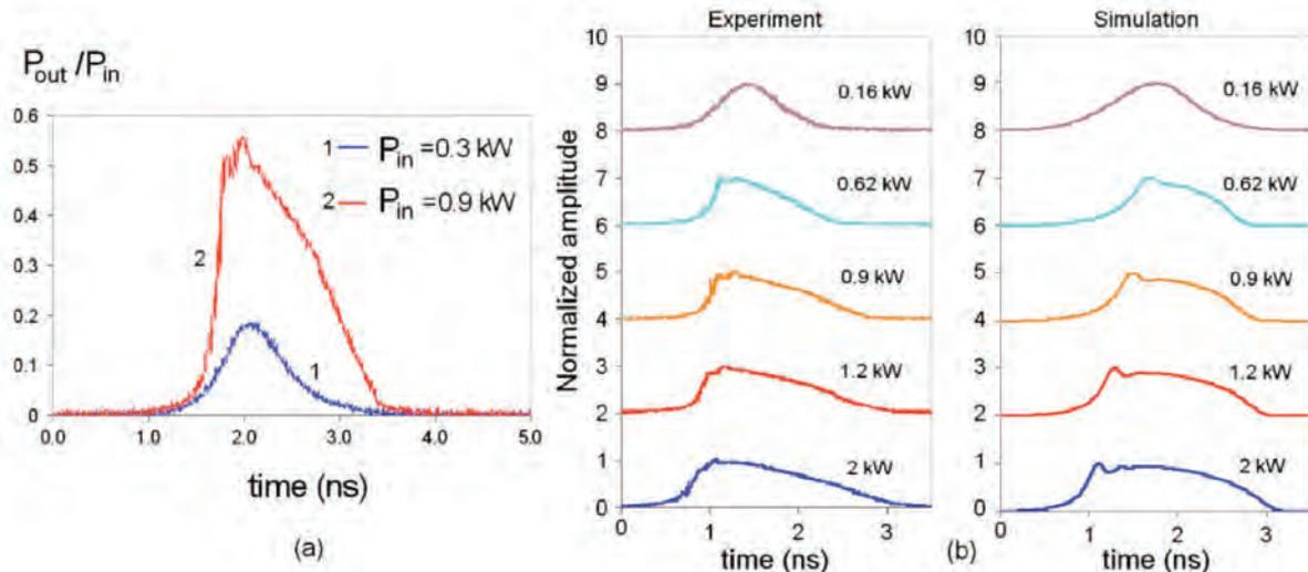
**Fig 4: (a) transmission (normalized to the input) versus time at low intensities (blue) and high intensities (red). (b) measured normalized transmissions for different power levels (c) calculated normalized transmissions for different power levels.**
