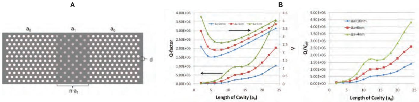
**Fig 2: (a) Heterostructure cavity.**  $a_0$  is period of PhC.  $\Delta a = a_1 - a_0$  is the constant shift of cavity,  $a_1$  is the period of cavity parallel to the waveguide direction. (b) The Q-factor and mode volume  $V$ . (c) The  $Q/V_{\text{eff}}$  ratio.
